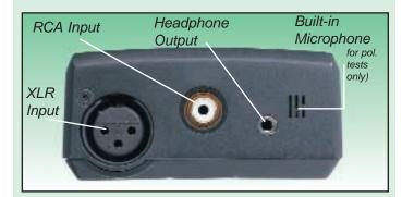
A balanced XLR as well as an unbalanced RCA connector are available to connect the test signal to the device. The system automatically detects the input source, while a headphone output allows monitoring of the input signal at a normalized level for aural diagnostics. A built-in microphone is provided for polarity checks. Broken connections in an XLR can easily be detected by the balance indicator.
